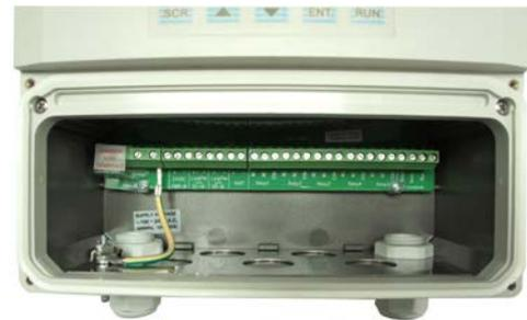
Figure 1 Terminal access on the LST400
